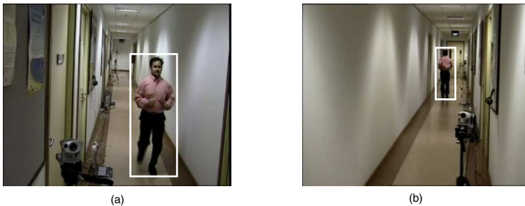
Fig. 3. An example: Bounding rectangles along the detected blobs in the video frames of (a) Camera 1 and (b) Camera 2, corresponding to a hummas “running” event
