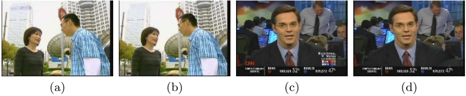
Fig. 3. Examples of TV logo removal based on the regularization PDE. (a) and (c) are original frames with TV logos. (b) and (d) are frames with removed TV logos.
