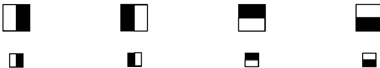
Fig. 5. The pattern codebook of four regular shaped, 128-pixel patterns, defined in 16x16 blocks in top row and 16-pixel patterns defined in 8x8 blocks in bottom row, where the white region represents 1 (motion) and black region represents 0 (no motion)
