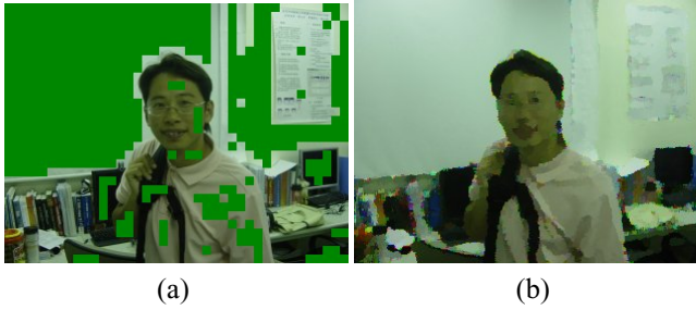
Fig. 7. (a) sum of AC^2 in green blocks < 1000 (b) applying oil-paint effect selectively
