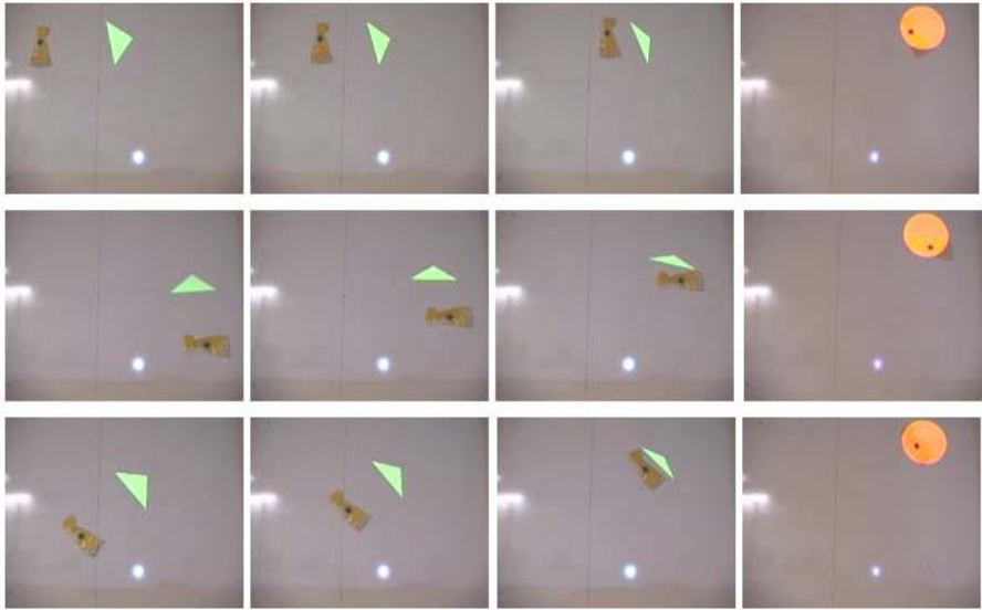
Fig. 3. Objects are placed at different start point but eventually get to the same destination point (the circle in the picture). The pictures should be viewed from left to right, top to bottom.
