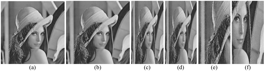
Fig. 2. Results of the proposed (2, 4) enhanced solution with \{p_0, p_1, p_2, p_3\}=\{17, 61, 67, 131\} using the image Lena:(a) 512×512 original image; (b) restored image with PSNR 48.88 dB obtained using two 256×512 shadow images shown in (c)-(d); (e)-(f) enlarged parts of the image shown in (d)
