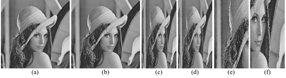
Fig. 1. Results of the proposed (2, 4) basic solution with \{p_0, p_1, p_2, p_3\}=\{17, 61, 131, 251\} using the image Lena: (a) 512×512 original image; (b) restored image with PSNR 50.53 dB obtained using two 256×512 shadow images shown in (c)-(d); (e)-(f) enlarged parts of the image shown in (d)
