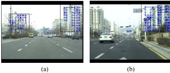
Fig. 10. (a) Example of false positive (FP). Left rectangle was falsely detected. (b) Example of false negative (FN). Buildings on the left side were not detected.
