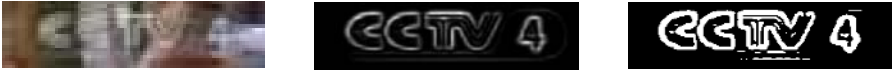
Fig. 2. TV logo mask extraction (Left to right: a frame from the original sequence, the generalized gradient image, and the logo's binary mask by OTSU algorithm)
