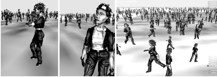
Fig. 1. Cached hardware skinning with geometry instancing for real time rendering of 1000 animated 3D humanoids. Judicious placement and cycle-time offsets of clones minimizes perceivable repetition. Character model and animation cycles sourced from [12].
